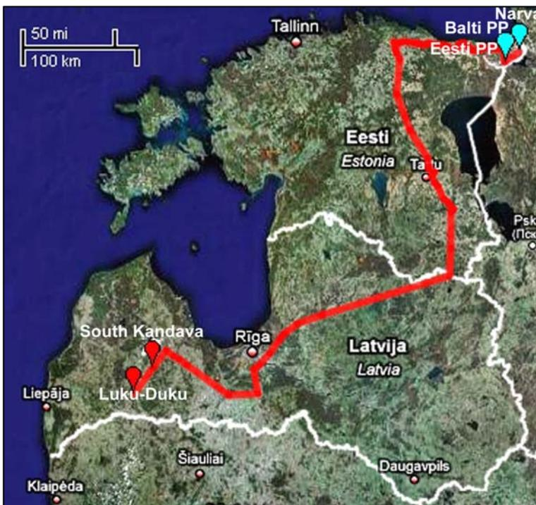
Figure 1 Estonian–Latvian case study. Eesti and Balti Power Plants are shown by green–blue symbols, storage sites by red symbols. The proposed CO<sub>2</sub> pipelines (along with natural gas pipelines) are shown by a red line.
